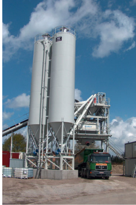
Mobil beton santrali (Fotoğraf:AWV PDe Winne)
