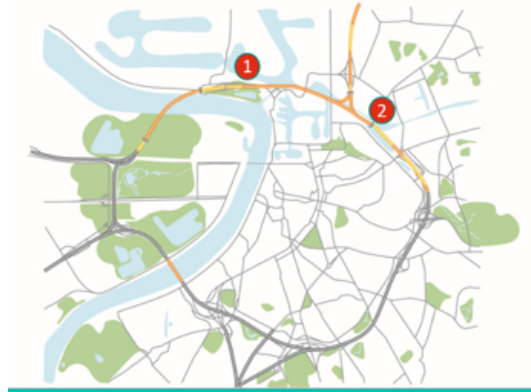
Figure 13. The Oosterweel link, completing the unfinished Ring Road with a new set of tunnels and replacing the current Ring Road Viaduct by tunnels and open trenches to be covered over time
