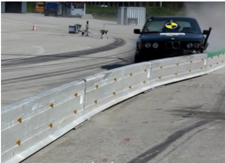
Figure 12. Flexible concrete system
