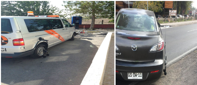
Figure 4. OBSI microphones for tire-pavement noise in Turkey and Chile
