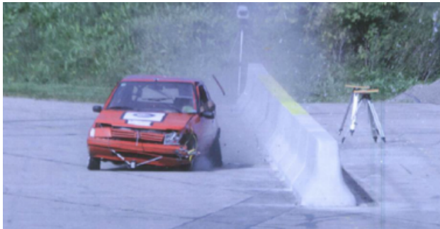
Figure 9. the EN 1317, “TB11” test to determine impact severity
