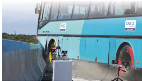
Figure 10. a TB51 test (13T, 70 km/h, 20°)
