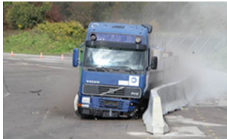
Figure 11. a TB81 test (38T, 65 km/h, 20°)
